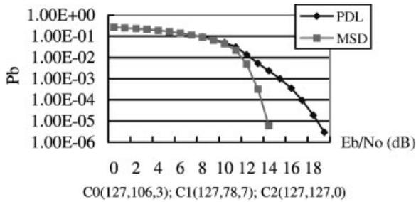
Fig. 21. Comparison of MLC/MSD and MLC/PDL with 8ASK, MP, over AWGN channel.
