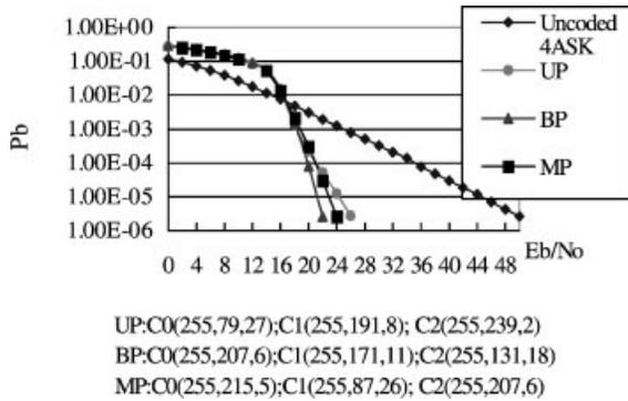
Fig. 12. Performance comparison of MLC/MSD with UP, BP and MP (Rayleigh channels).
