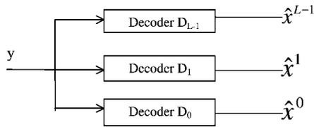
Fig. 4. Parallel decoding of levels (PDL).
