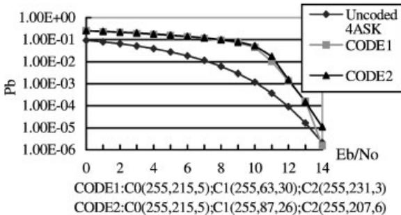
Fig. 18. Performance comparison of different rate design (AWGN channel, MP, MLC/MSD).
