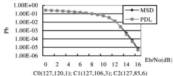
Fig. 20. Comparison of MLC/MSD and MLC/PDL with BP over AWGN channel.
