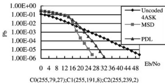
Fig. 22. Comparison of MLC/MSD and MLC/PDL with UP over Rayleigh channel.
