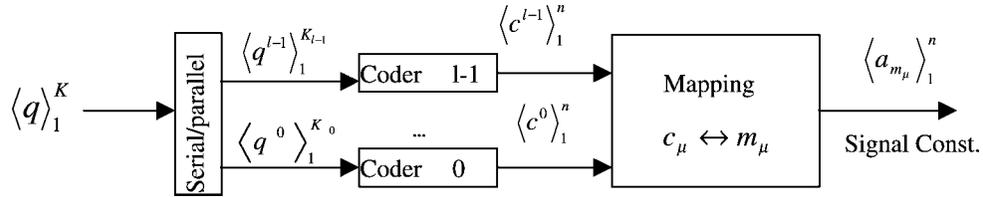
Fig. 1. Multilevel coding scheme.
