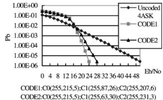
Fig. 15. Performance comparison of different rate design (Rayleigh channel, MP, MLC/MSD).
