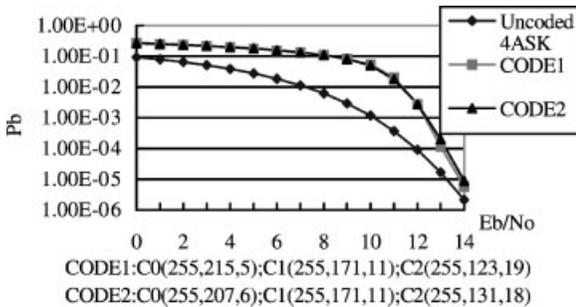
Fig. 17. Performance comparison of different rate design (AWGN channel, BP, MLC/MSD).
