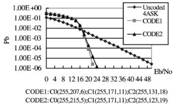
Fig. 14. Performance comparison of different rate design (Rayleigh channels, BP, MLC/MSD).
