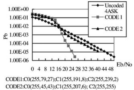
Fig. 13. Performance comparison of different rate design (Rayleigh channels, UP, MLC/MSD).
