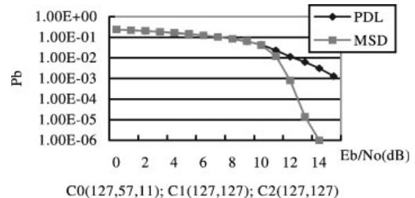
Fig. 19. Comparison of MLC/MSD and MLC/PDL with UP over AWGN channel.
