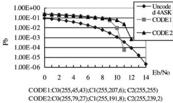
Fig. 16. Performance comparison of different rate design (AWGN channel, UP, MLC/MSD).
