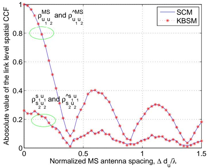
Fig. 4. The absolute values of the link level spatial CCFs of the SCM and KBSM with Gaussian subpath PASs ( $\Delta d_s/\lambda = 1$ ,  $\theta_{BS} = 50^0$ ,  $\theta_{MS} = 195^0$ , BS AS =  $5^0$ , MS AS =  $35^0$ ).
