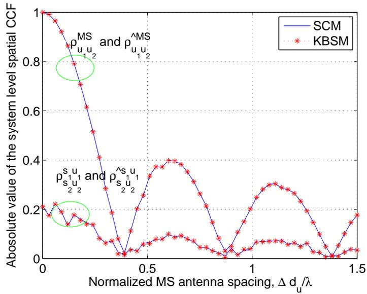
Fig. 5. The absolute values of the system level spatial CCFs of the SCM and KBSM with Gaussian subpath PASs ( $\Delta d_s/\lambda = 1$ , BS AS =  $5^\circ$ , MS AS =  $35^\circ$ ).
