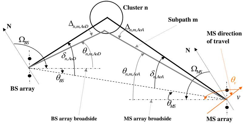
Fig. 1. BS and MS angle parameters in the 3GPP SCM with one cluster of scatterers [14].
