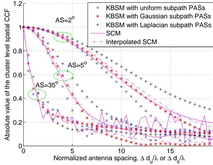
Fig. 2. The absolute values of the cluster level spatial CCFs of the SCM, interpolated SCM, and KBSMs with uniform, Gaussian, and Laplacian subpath PASs (mean AoA/AoD =  $60^\circ$ ).
