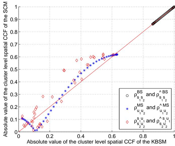
Fig. 3. The absolute values of the cluster level spatial CCFs of the SCM and KBSM with Gaussian subpath PASs ( $\Delta d_s/\lambda = 1$ ,  $\Delta d_u/\lambda = 1$ , BS AS =  $5^0$ , MS AS =  $35^0$ ).
