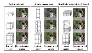
Fig. 5. Illustration of the latent representations of mask-based and/or residual-based DIC schemes. The encoding rate increases progressively from the first row to the third row. In the residual-based DIC scheme, extra available bits are used to add more layers in the latent space. In the spatial mask-based DIC scheme, extra bits are used to better encode spatially important regions.
