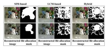
Fig. 4. Illustration of spatial mask-based bit allocation strategies. The white dots in the mask indicate areas where more bits are allocated; the first row has a higher rate than the second row.
