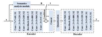
Fig. 8. Network structure of the MPGC-2 model. The vectors  ${\bf B}$  and  ${\bf 1}$  are separate inputs as conditional vectors during training.
