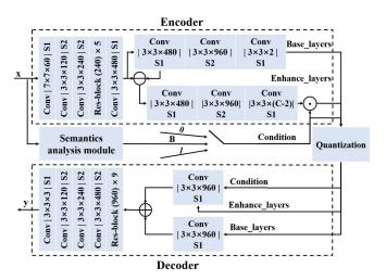
Fig. 10. Network structure of the RMPGC model. The vectors **B**, **0**, and **1** are separate inputs as conditional vectors during training.
