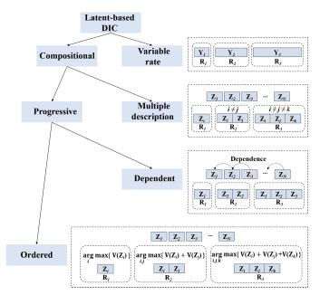
Fig. 2. Classification of latent-based variable-rate DIC schemes and illustration of their rate adaptation mechanisms ( $Z_i$  denotes different pieces of data after encoding,  $R_i$  denotes different rates of data packet encapsulation,  $V(Z_i)$  is a function that marks the importance of data piece  $Z_i$  with respect to certain context).
