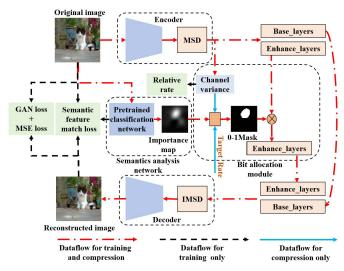
Fig. 9. The framework of the RMPGC algorithm. The rectangle orange block represents the mask-based bits allocation module, which generates a binary mask according to the target rate,  $C_b$ , LCM, and SIM.
