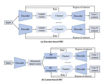
Fig. 1. Two architectures of rate adaptive DIC: (a) encoder-based architecture; (b) latent-based architecture.
