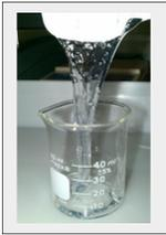
Fig. 1: An aqueous solution of 10% by weight PVA in water.
