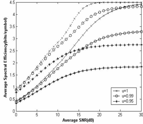
Fig. 5. Average spectral efficiency versus the average SNR for different  $u$  ( $N_r = 1$ , dashed line:  $N_T = 2, N_R = 2$ ; solid line:  $N_T = 1, N_R = 1$ )
