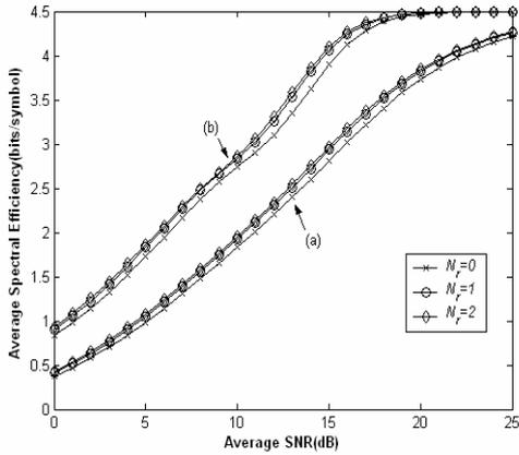
Fig. 3. Average spectral efficiency versus the average SNR for different retransmission numbers with the perfect channel estimation (a)  $N_T = 1, N_R = 1$  (b)  $N_T = 2, N_R = 2$ .
