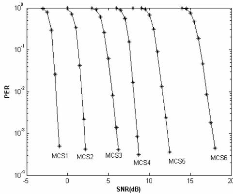
Fig. 2. PER simulation performance and fitting curves of six MCSs (star: simulation; solid line: fitting curve).
