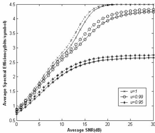
Fig. 4. Average spectral efficiency versus the average SNR for different  $u$  (dashed line:  $N_r = 1$ ; solid line:  $N_r = 0$ ;  $N_T = 2, N_R = 2$ ).
