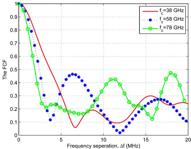
Fig. 8. The FCFs of the proposed simulation channel model at different frequencies  $f_c$  ( $D_{pn,m_n}^T(t_0) = 50$  m,  $D_{qn,m_n}^R(t_0) = 100$  m,  $\lambda_G = 80$  m,  $\lambda_R = 4$  m,  $v_R = 100$  m/s).
