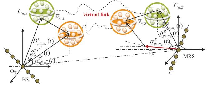
Fig. 2. A 3D non-stationary twin-cluster HST channel model.
