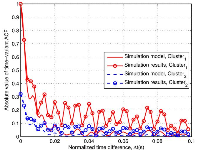
Fig. 7. The comparison of time-variant ACFs of simulation model and simulation results ( $f_c = 58$  GHz,  $D_{p_n, m_n}^T(t_0) = 50$  m,  $D_{q_n, m_n}^R(t_0) = 100$  m,  $\lambda_G = 80$  m,  $\lambda_R = 4$  m,  $v_{n,A} = 30$  m/s,  $v_{n,Z} = 30$  m/s,  $v_R = 100$  m/s).
