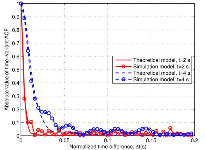
Fig. 6. The time-variant ACFs of the theoretical model and simulation model ( $f_c = 58$  GHz,  $D_{p_n, m_n}^T(t_0) = 50$  m,  $D_{q_n, m_n}^R(t_0) = 100$  m,  $\lambda_G = 80$  m,  $\lambda_R = 4$  m,  $v_{n,A} = 30$  m/s,  $v_{n,Z} = 30$  m/s,  $v_R = 100$  m/s).
