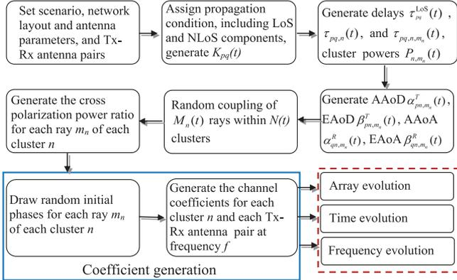
Fig. 3. The generation process of the HST channel model.
