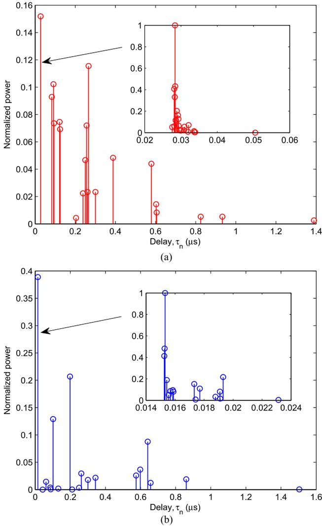
Fig. 5. The delay PSDs of the non-stationary HST simulation channel model at (a)  $t = 2$  s and (b)  $t = 4$  s ( $D_{p_n, m_n}^T(t_0) = 50$  m,  $D_{q_n, m_n}^R(t_0) = 100$  m,  $\lambda_G = 80$  m,  $\lambda_R = 4$  m,  $v_{n,A} = 30$  m/s,  $v_{n,Z} = 30$  m/s,  $v_R = 100$  m/s).
