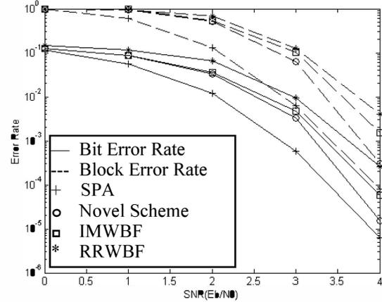
Figure 1: Bit error rate (solid line) and block error rate (dashed line) performances for different WBF methods on the (273,191) PG-LDPC code
