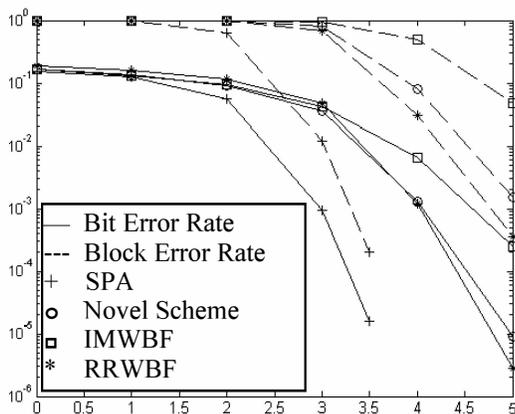
Figure 2: Bit error rate (solid line) and block error rate (dashed line) performances for different WBF methods on the (816,408) LDPC code
