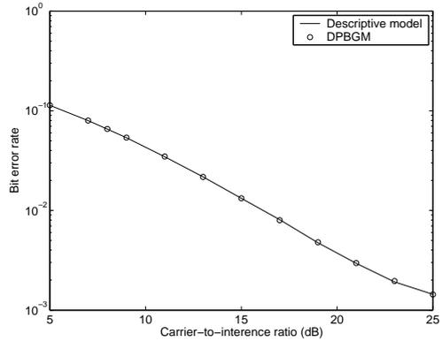
Fig. 2: The BERs of the uncoded EGPRS system with the TU3 IFH channel obtained from the descriptive model and the DPBGM.
