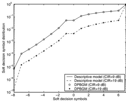
Fig. 5: The soft decision symbol distributions for the descriptive model and the DPBGM (CIR=9 dB and CIR=19 dB).
