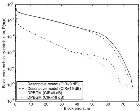
Fig. 4: The block error probability distributions of the descriptive model and the DPBGM (CIR=9 dB and CIR=19 dB).
