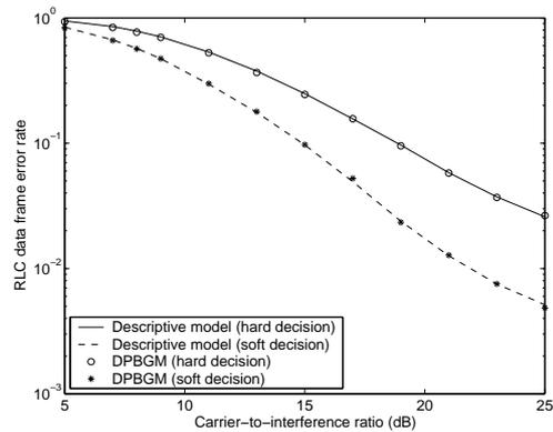
Fig. 6: The RLC data FERs of the coded EGPRS system with hard and soft decision decoding algorithms obtained from the descriptive model and the DPBGM.
