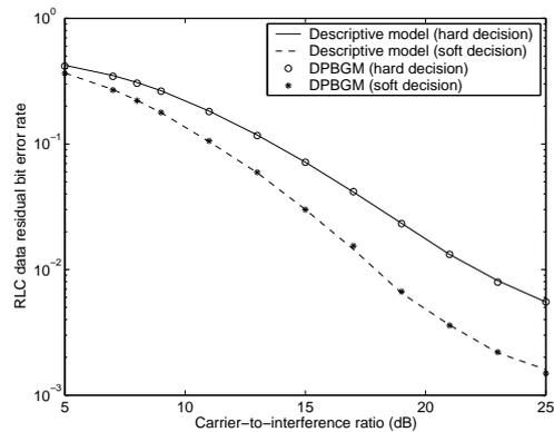
Fig. 7: The RLC data RBERs of the coded EGPRS system with hard and soft decision decoding algorithms obtained from the descriptive model and the DPBGM.
