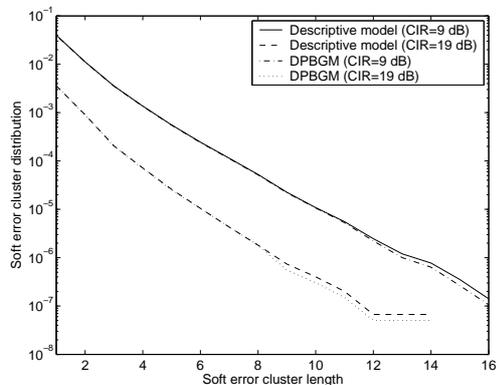
Fig. 3: The soft error cluster distributions of the descriptive model and the DPBGM (CIR=9 dB and CIR=19 dB).
