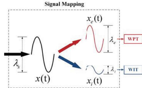
Fig. 2. The signal mapping splits the received signal  $x(t)$  into information signal  $x_i(t)$  and the energy signal  $x_e(t)$ .
