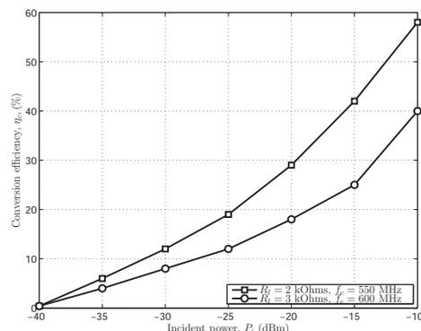
Fig. 4. The CE-IP relation in a DTV signal harvesting system. A load circuit is used to evaluate the system performance in the proposed system [9].
