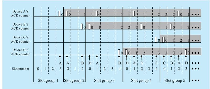
**Fig.2** The transition period from contention-based random access to contention-free deterministic access in a four-device network.
