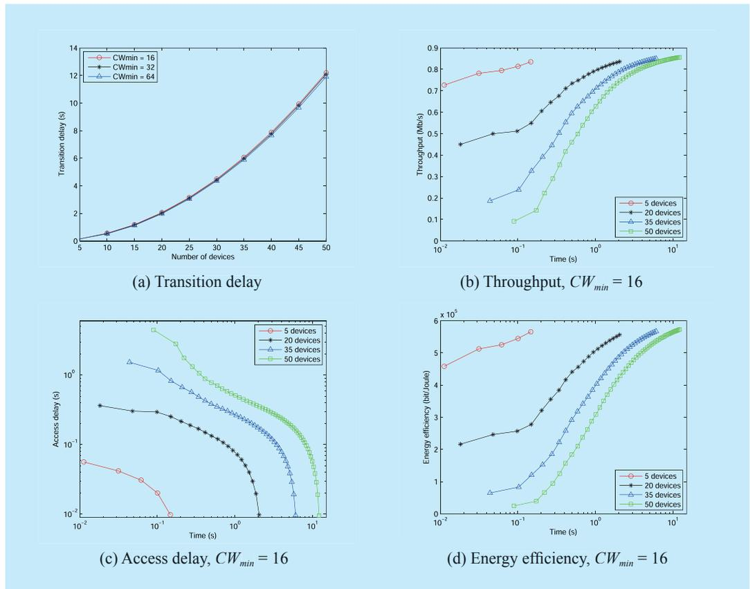
**Fig.3** Transition delay, throughput, access delay and energy efficiency of NAMA in transition period,  $CW_{max} = 1024$
