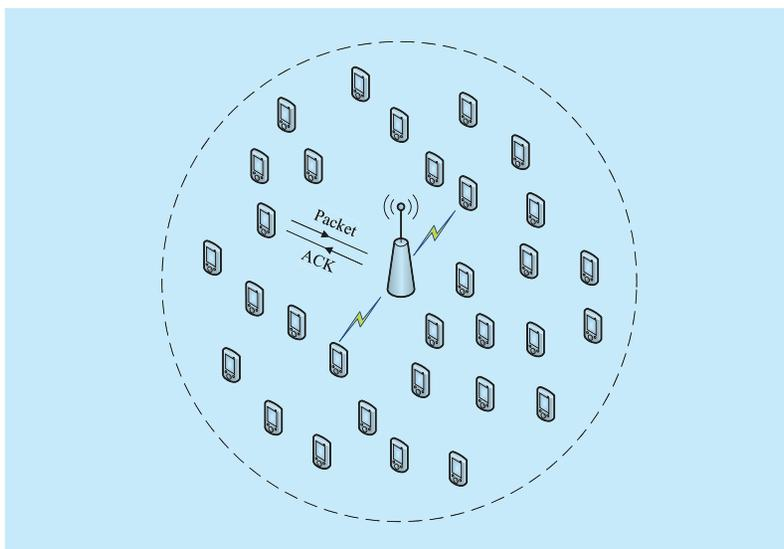
Fig.1 A typical contention-based network.
