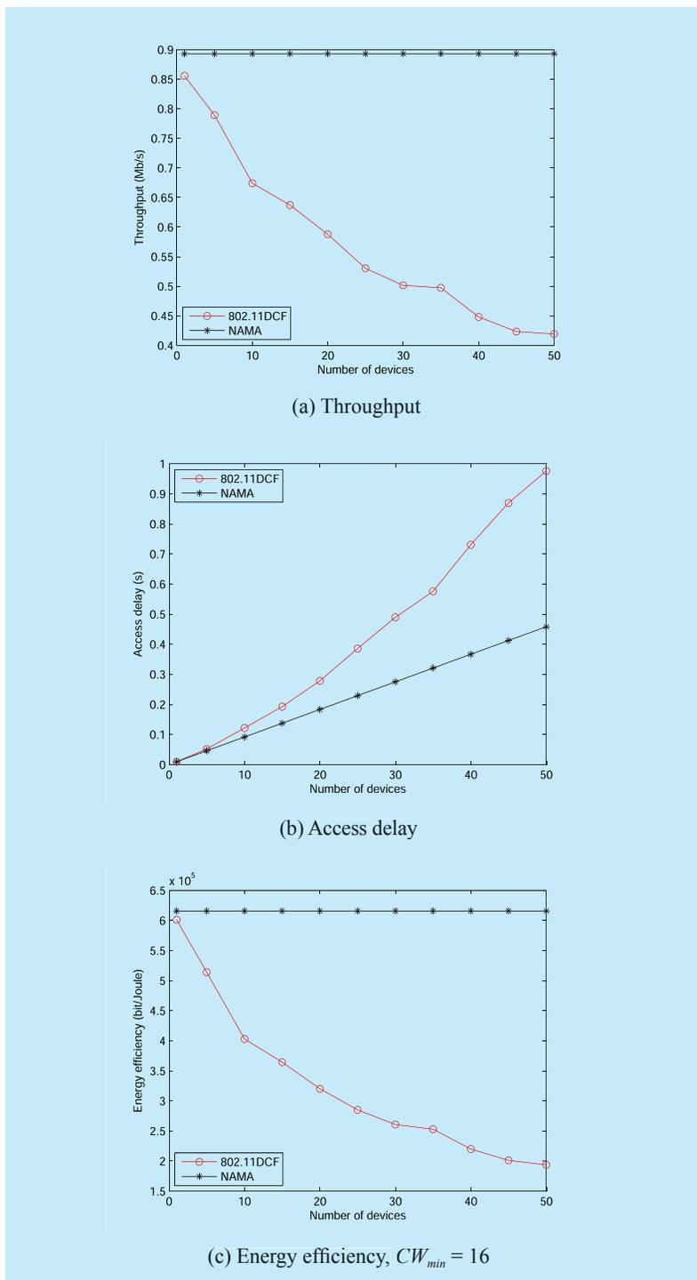
**Fig.4** Throughput, access delay and energy efficiency of NAMA in deterministic state,  $CW_{min} = 16$ ,  $CW_{max} = 1024$ .
