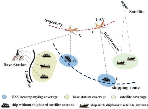
Fig. 1. Illustration of a hybrid satellite-UAV-terrestrial maritime communication network, where grey dotted lines denote wireless communication links.
