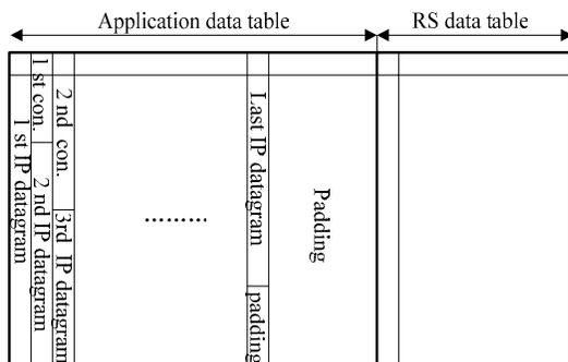
Fig. 4. The structure of a GSE-FEC frame.
