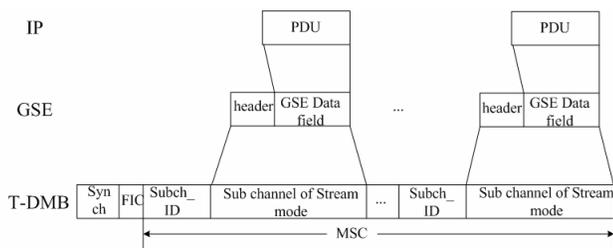
Fig. 2. GSE within the T-DMB protocol stack.
