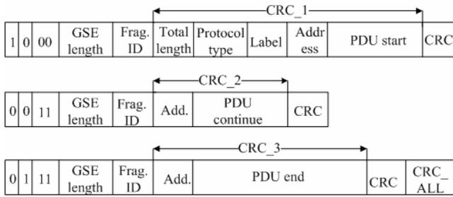
Fig. 6. The CRC scheme for a fragmented PDU.
