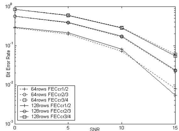
Fig. 9. Bit Error Rates after GSE-FEC with NE decoding.
