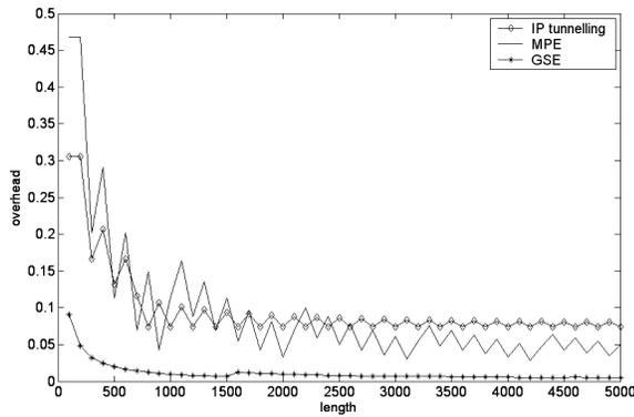
Fig. 3. The overheads of IP tunneling, MPE and GSE.
