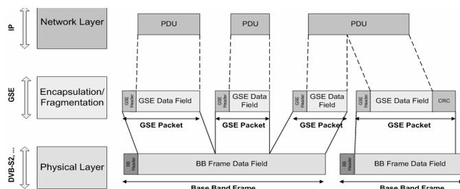
Fig.1. GSE within the DVB protocol stack.
