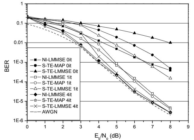
Fig. 6. Comparison of the BER performance between NI-LMMSE, S-TE-MAP and S-TE-LMMSE for the BPSK modulation and the ISI channel  $M=3$ .
