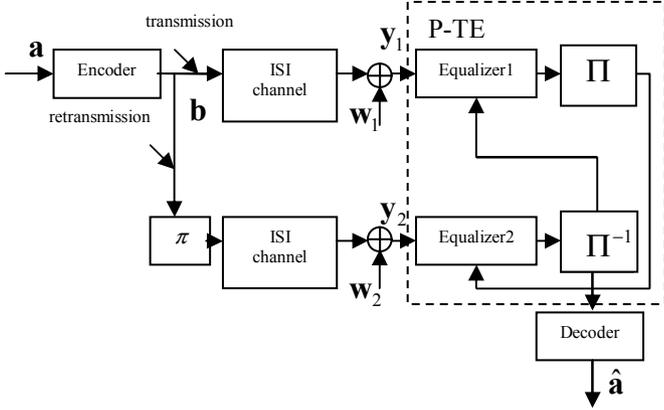
Fig. 2. A coded data transmission system with a P-TE.
