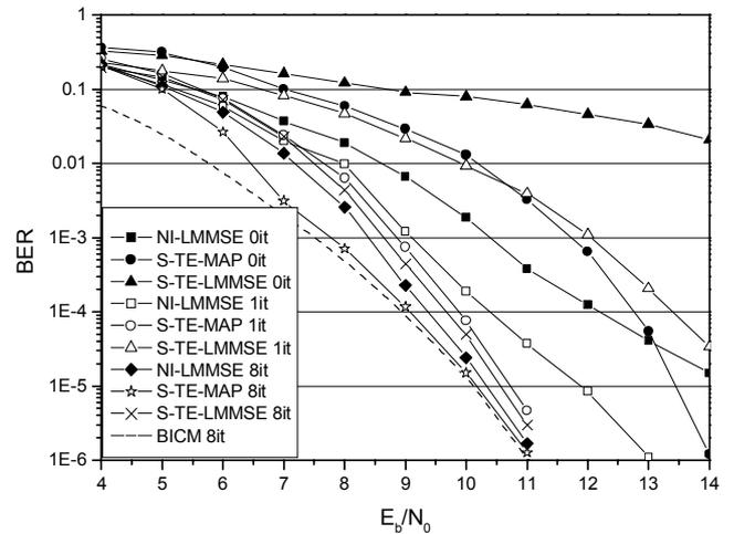
Fig. 7. Comparisons of the BER performance of NI-LMMSE, S-TE-MAP, and S-TE-LMMSE for the 8PSK modulation and the ISI channel  $M=5$ .
