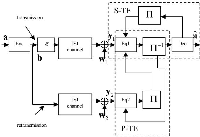
Fig. 3. A coded data transmission system with a novel iterative method for TE.
