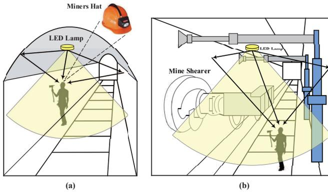
Fig. 1. System model, (a) Horseshoe mining roadway, (b) Mine working face.
