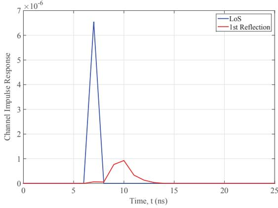
Fig. 4. Channel impulse response in mining roadway.
