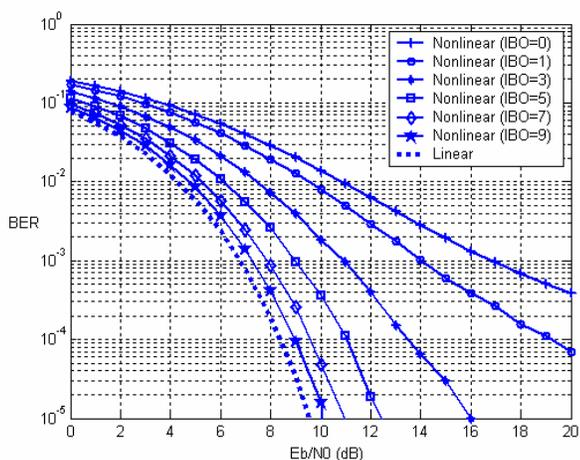
Fig. 5. BER of MC-CDMA using SSPA with different IBO
