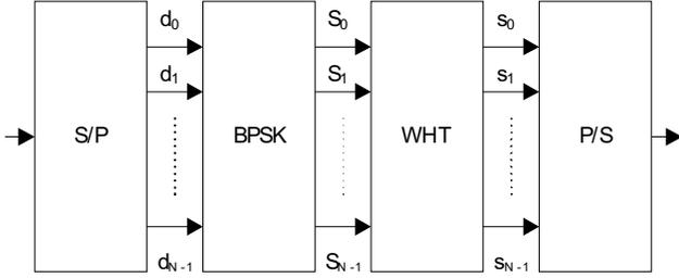
Fig. 1. Simplified block diagram of the MC-CDMA transmitter.
