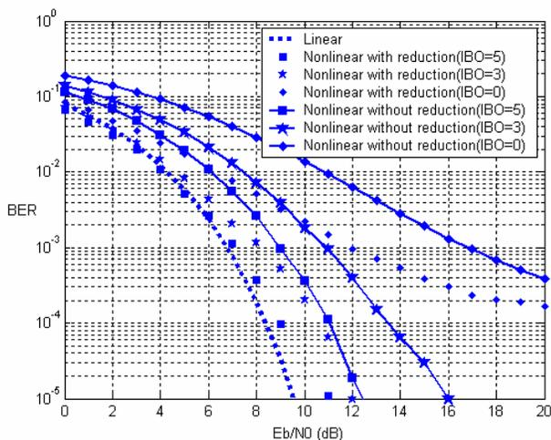
Fig. 6. BER before and after PAPR reduction in SSPA
