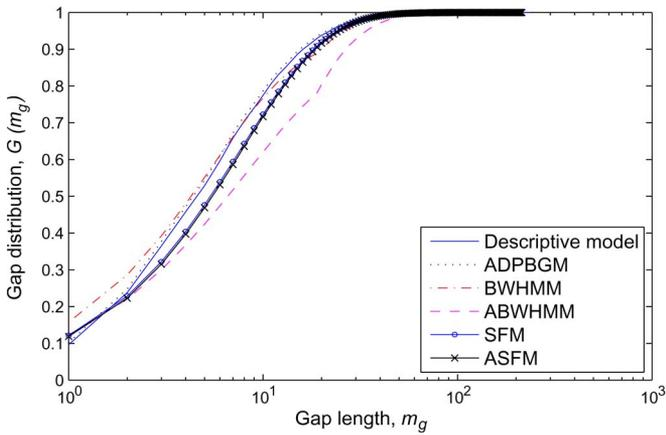
Fig. 7. The GDs of the descriptive model, generative models, and three adaptive generative models (SNR = 4 dB obtained from 3 dB and 5 dB).
