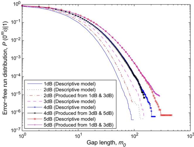
Fig. 1. The EFRDs of the descriptive model for several SNRs and reproduced EFRDs.
