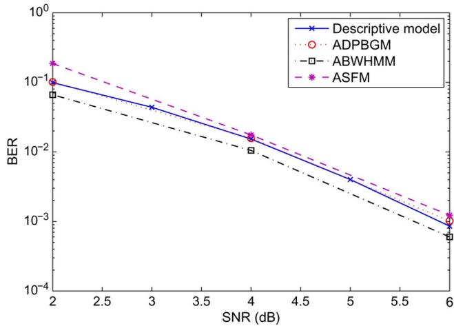
Fig. 12. The coded BER of the descriptive model and three adaptive generative models.
