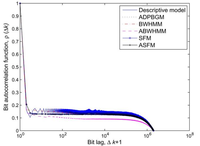
Fig. 5. The BECFs of the descriptive model, generative models, and three adaptive generative models (SNR = 4 dB obtained from 3 dB and 5 dB).
