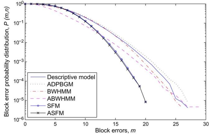
Fig. 4. The BEPDs of the descriptive model, generative models, and three adaptive generative models (SNR = 4 dB obtained from 3 dB and 5 dB,  $n = 50$ ).
