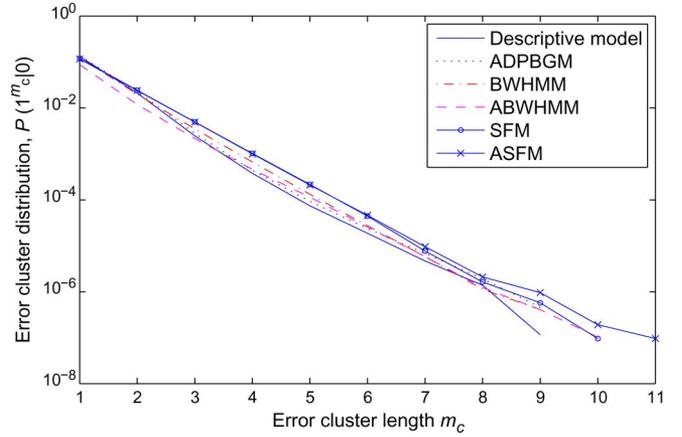
Fig. 3. The ECDs of the descriptive model, generative models, and three adaptive generative models (SNR = 4 dB obtained from 3 dB and 5 dB).
