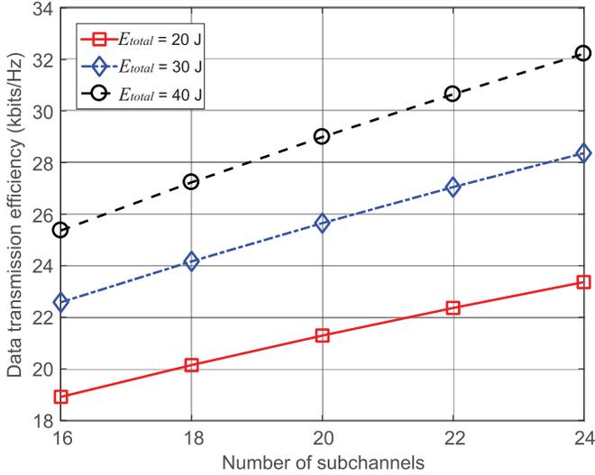
Fig. 8. The relationship between the overall data transmission efficiency and the number of subchannels, where the proposed Algorithm 3 is used.
