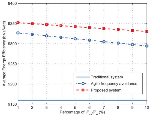
Fig. 5. The average energy efficiency of different PLC systems when the signal detection power  $P_{ss}$  varies. The probability of the interference occurring is  $\Pr(\mathcal{H}_{1,n}) = 0.3$ , and the average transmit power constraint is  $\Gamma_n = 40$  dBm.
