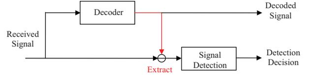
Fig. 2. Receiver structure of the proposed green data transmission PLC system.
