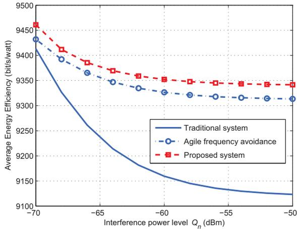
Fig. 4. The average energy efficiency of different PLC systems when the interference power level  $Q_n$  varies. The probability of the interference occurring is  $\Pr(\mathcal{H}_{1,n}) = 0.3$ , while the average transmit power constraint is set to be  $\Gamma_n = 40$  dBm.
