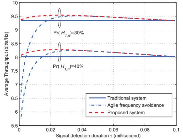
Fig. 3. The relation between the signal detection duration  $\tau$  and the average throughput for different PLC systems. The influence of the probability of interference occurring is also shown. The average transmit power constraint is  $\Gamma_n = 40$  dBm.
