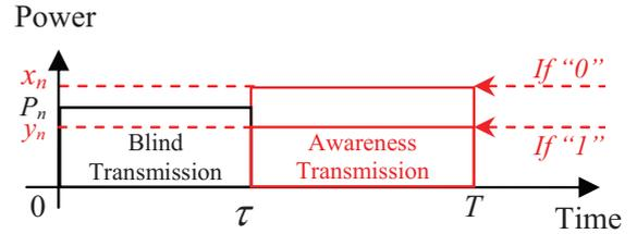
Fig. 1. Frame structure of the proposed green data transmission PLC system.
