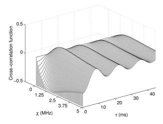
Fig. 4: Cross-correlation function  $r_{\mu_1\mu'_2}(\tau,\chi)$ (ref. model) for the COST 207 RA profile ( $\alpha = 0.1086 \ \mu s, f_{max} = 91 \ Hz, \sigma_0^2 = 1$ ).
