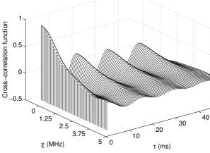
Fig. 3: Cross-correlation function  $\hat{r}_{\mu_i\mu'_i}(\tau,\chi)$ (sim. model, N = 20, M = 20) for the COST 207 RA profile ( $\alpha = 0.1086 \ \mu s$ ,  $f_{max} = 91$  Hz,  $\sigma_0^2 = 1$ ).
