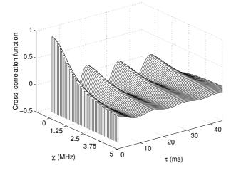
Fig. 2: Cross-correlation function  $r_{\mu_i\mu'_i}(\tau,\chi)$ (ref. model) for the COST 207 RA profile ( $\alpha = 0.1086 \ \mu s, f_{max} = 91 \ Hz, \sigma_0^2 = 1$ ).
