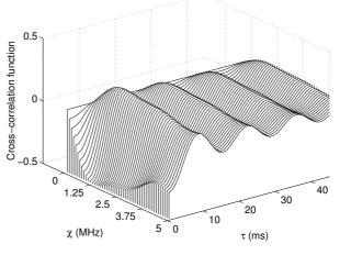
Fig. 5: Cross-correlation function  $\hat{r}_{\mu_1\mu'_2}(\tau, \chi)$ (sim. model, N = 20, M = 20) for the COST 207 RA profile ( $\alpha = 0.1086 \ \mu s$ ,  $f_{max} = 91$  Hz,  $\sigma_0^2 = 1$ ).
