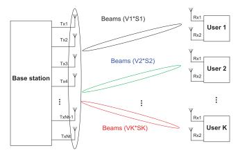
FIGURE 2. Block diagram of a BD-MU-SM system.
