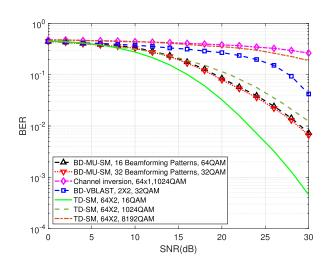
**FIGURE 11.** BER performance of different systems with 16 users,  $\beta = 0.3$ , data rate = 10 bits/symbol/user.
