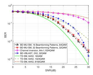
**FIGURE 9.** BER performance of different systems with 4 users,  $\beta = 0.3$ , data rate = 10 bits/symbol/user.
