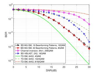
**FIGURE 10.** BER performance of different systems with 16 users,  $\beta = 0.3$ , data rate = 8 bits/symbol/user.
