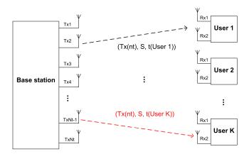
FIGURE 1. Block diagram of a TDMA-MU-SM system.
