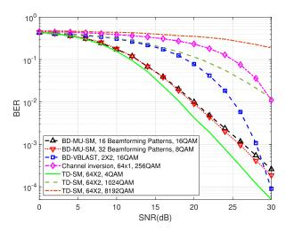
**FIGURE 8.** BER performance of different systems with 4 users,  $\beta = 0.3$ , data rate = 8 bits/symbol/user.
