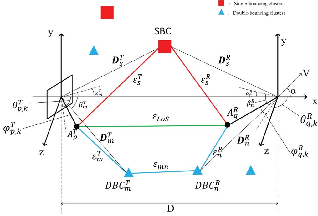
Fig. 1. mmWave massive MIMO communication system with angular parameters and single- and double-bouncing scattering propagation.
