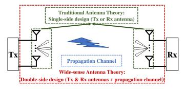
Fig. 5. The description of the traditional antenna theory and wide-sense antenna theory.
