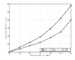
Fig. 4. The CE-IP relation in a DTV signal harvesting system. A load circuit is used to evaluate the system performance in the proposed system [9].
