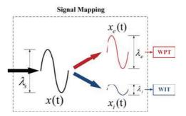
Fig. 2. The signal mapping splits the received signal x(t) into information signal  $x_i(t)$  and the energy signal  $x_e(t)$ .
