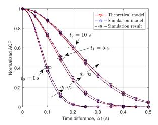
Fig. 5. The comparison of time-variant ACFs of theoretical model, simulation model, and simulation results for cluster  $C_1^{\rm S}$  at  $t_0=0$  s,  $t_1=5$  s and  $t_2=10$  s with  $q_1=1$  and  $q_2=200$  (D=3 m, p=1,  $f_0=325$  GHz,  ${\bf v}^{\rm R}=0.1$  m/s,  $\zeta^{\rm R}=0,\xi^{\rm R}=\frac{\pi}{3},\mu_{c,\theta}^{\rm SR}=1.4^\circ,\mu_{c,\phi}^{\rm SR}=2.8^\circ,r_c^{\rm CT}=0.4$ ).
