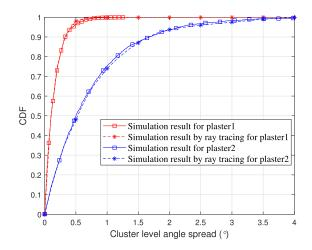
Fig. 10. The comparison of cluster level angular spread with different materials ( $p=1,\,q=1,\,t_0=0$  s,  $f_0=300$  GHz,  ${\bf v}^{\bf R}=0$  m/s,  $r_c^{\bf ST}=0.4,\,\mu_{c,\phi}^{\bf SR}=0.15^\circ$  for plaster1,  $\mu_{c,\phi}^{\bf SR}=0.75^\circ$  for plaster2).
