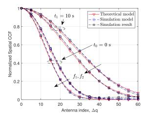
Fig. 6. The comparison of spatial CCFs of theoretical model, simulation model, and simulation results for cluster  $C_1^{\rm S}$  (D=3 m, p=1, q=1,  $t_0=0$  s,  $t_1=10$  s,  $f_1=300$  GHz,  $f_2=350$  GHz,  ${\bf v}^{\rm R}=0.1$  m/s,  ${\bf \zeta}^{\rm R}=0$ ,  ${\bf \xi}^{\rm R}=\frac{\pi}{3}$ ,  ${\bf \alpha}^{\rm R}=\frac{\pi}{3}$ ,  ${\bf \beta}^{\rm R}=\frac{\pi}{4}$ ,  $\mu_{c,\theta}^{\rm SR}=1.4^{\circ}$ ,  $\mu_{c,\phi}^{\rm SR}=2.8^{\circ}$ ,  $r_c^{\rm ST}=0.4$ ).
