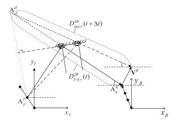
Fig. 2. Geometric relationship of the time-variant path via the SBC.
