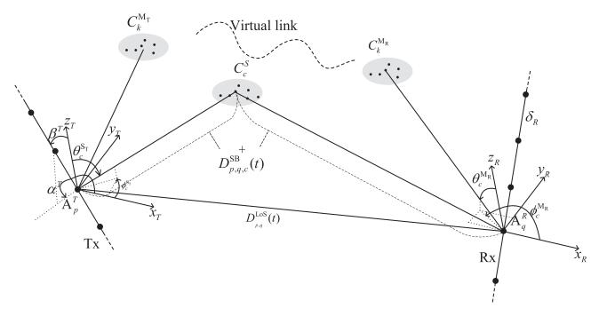
Fig. 1. A 3D THz GBSM for massive MIMO communication systems.
