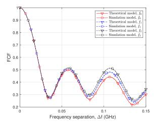
Fig. 7. The comparison of FCFs of theoretical model and simulation model at  $f_0=300$  GHz,  $f_1=325$  GHz and  $f_2=350$  GHz (D=3 m, p=1, q=1,  $t_0=0$  s,  ${\bf v^R}=0$  m/s,  $\mu^{\rm S_T}_{c,\theta}=1.2^\circ,$   $\mu^{\rm S_T}_{c,\phi}=1.7^\circ,$   $\mu^{\rm S_R}_{c,\theta}=1.4^\circ,$   $\mu^{\rm S_R}_{c,\phi}=2.8^\circ,$   $\mu^{\rm TOA}_{c}=0.3$  ns,  $\rho^{\rm S_T}_{\phi}=\rho^{\rm S_T}_{\varphi}=\rho^{\rm S_R}_{\phi}=\rho^{\rm S_R}_{\varphi}=1.2).$
