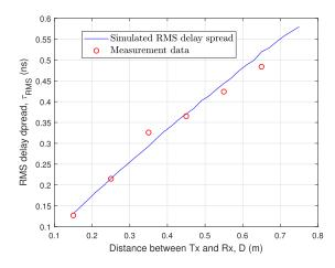
Fig. 11. The comparison of simulated RMS delay spread and measurement in [50]  $(p=1,\,q=1,\,t_0=0~{\rm s},\,f_0=300~{\rm GHz},\,{\rm v^R}=0~{\rm m/s},\,\mu_{\Delta\tau_{\rm SB}}=0.08,\,\mu_{\Delta\tau_{\rm MB}}=0.07~{\rm for}~D=0.15~{\rm m}).$
