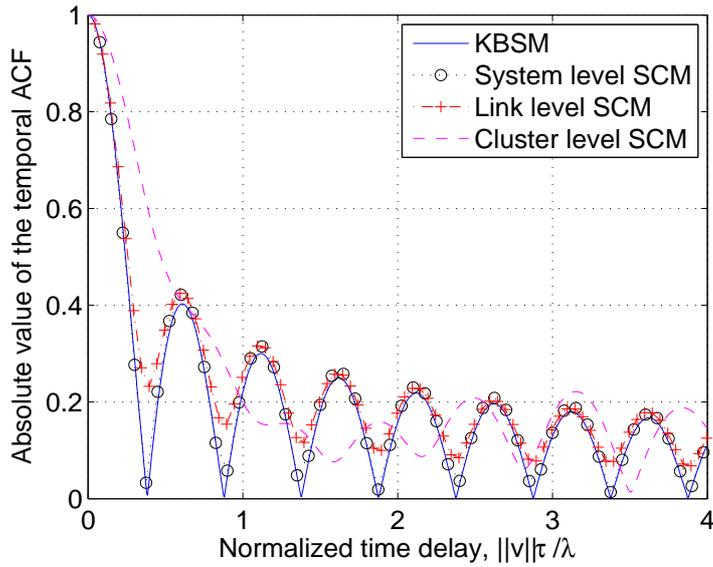
Fig. 6. The absolute values of the temporal ACFs of the KBSM and SCM at the cluster level, link level, and system level ( $\theta_v = 60^\circ$ ).
