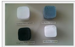
Fig. 2: PVA-C TMM after 4 freeze-thaw cycles samples for control, silicon carbide (SiC), graphite and aluminium oxide (AlO).
