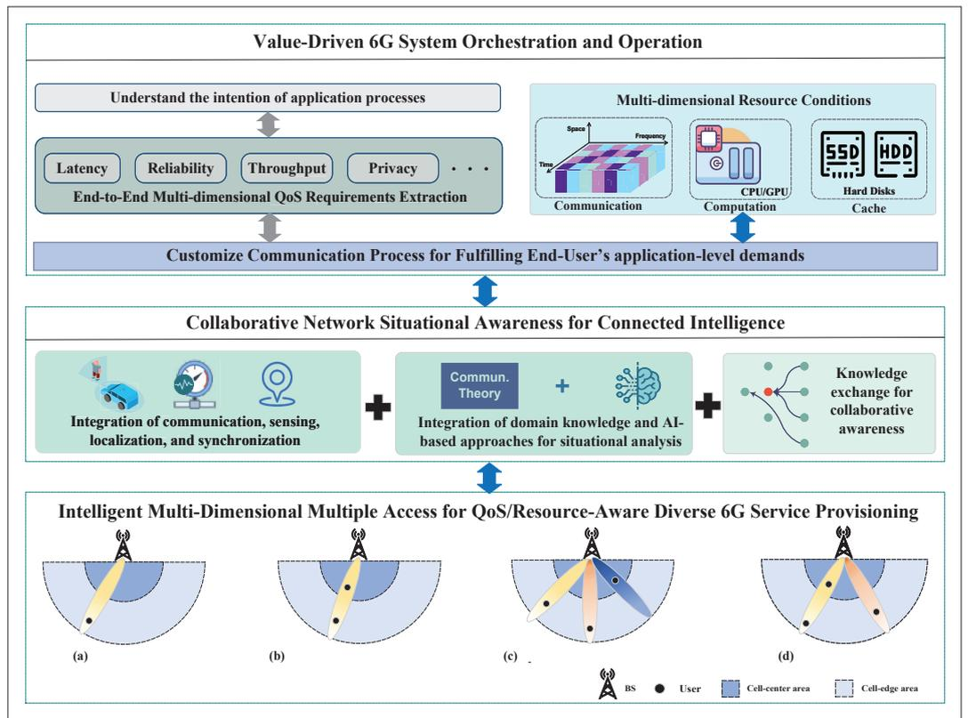
FIGURE 2. The illustration of key enabling technologies for value-oriented 6G systems. Value-driven 6G system orchestration and operation automatically transforms end-user's specific requirements at application-level into individualized QoS requirements. Then, with collaborative network situational awareness, intelligent multi-dimensional multiple access are utilized to fulfill user's specific QoS requirements.
