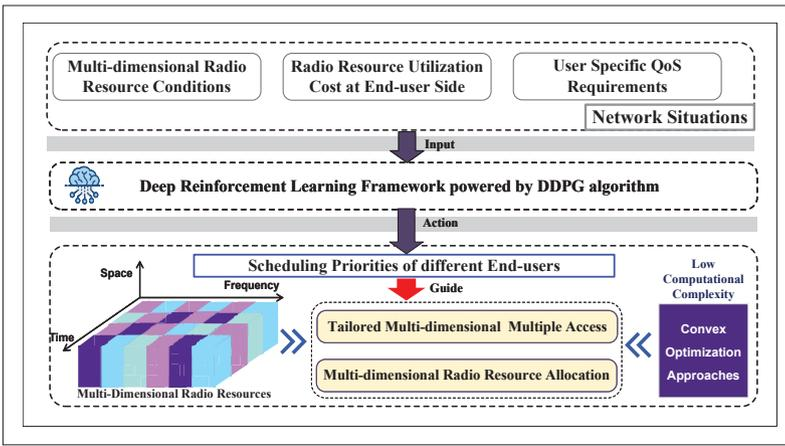
FIGURE 3. An illustration of the proposed value-oriented 6G MDMA scheme in the simulation.
