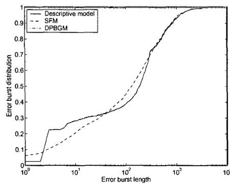
Fig. 6. The error burst distributions of the generative models and the descriptive model.
