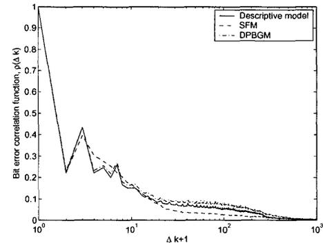
Fig. 8. The bit error correlation functions of the generative models and the descriptive model
