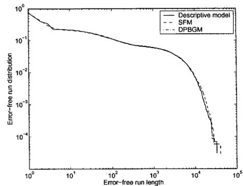
Fig. 4. The error-free run distributions of the generative models and the descriptive model.
