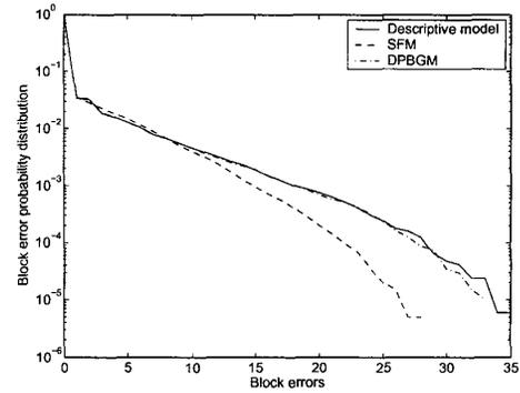
Fig. 7. The block error probability distributions of the generative models and the descriptive model.
