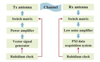
Fig. 1. System chart of the ultra-massive MIMO channel sounder.
