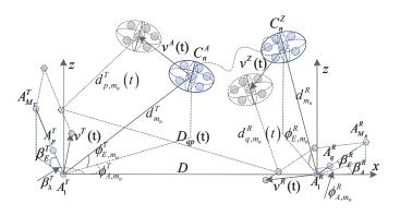
Fig. 5. A general 3D ultra-massive MIMO GBSM for 6G communication systems.
