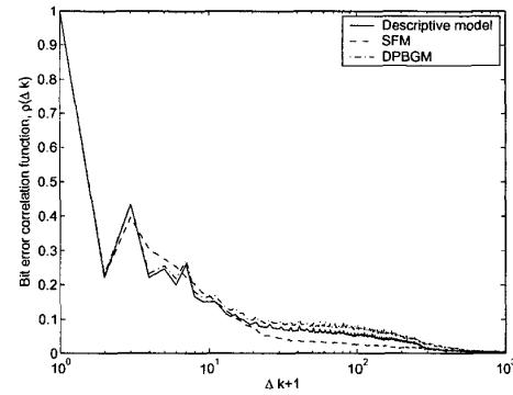
Fig. 8. The bit error correlation functions of the generative models and the descriptive model
