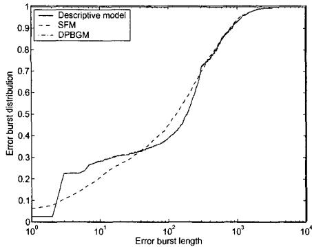
Fig. 6. The error burst distributions of the generative models and the descriptive model.
