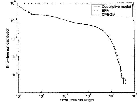
Fig. 4. The error-free run distributions of the generative models and the descriptive model.
