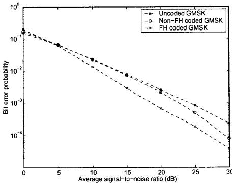
Fig. 2. Comparison of BEPs for uncoded GMSK (without interleaving and FH), non-FH coded GMSK (with interleaving), and FH coded GMSK systems.
