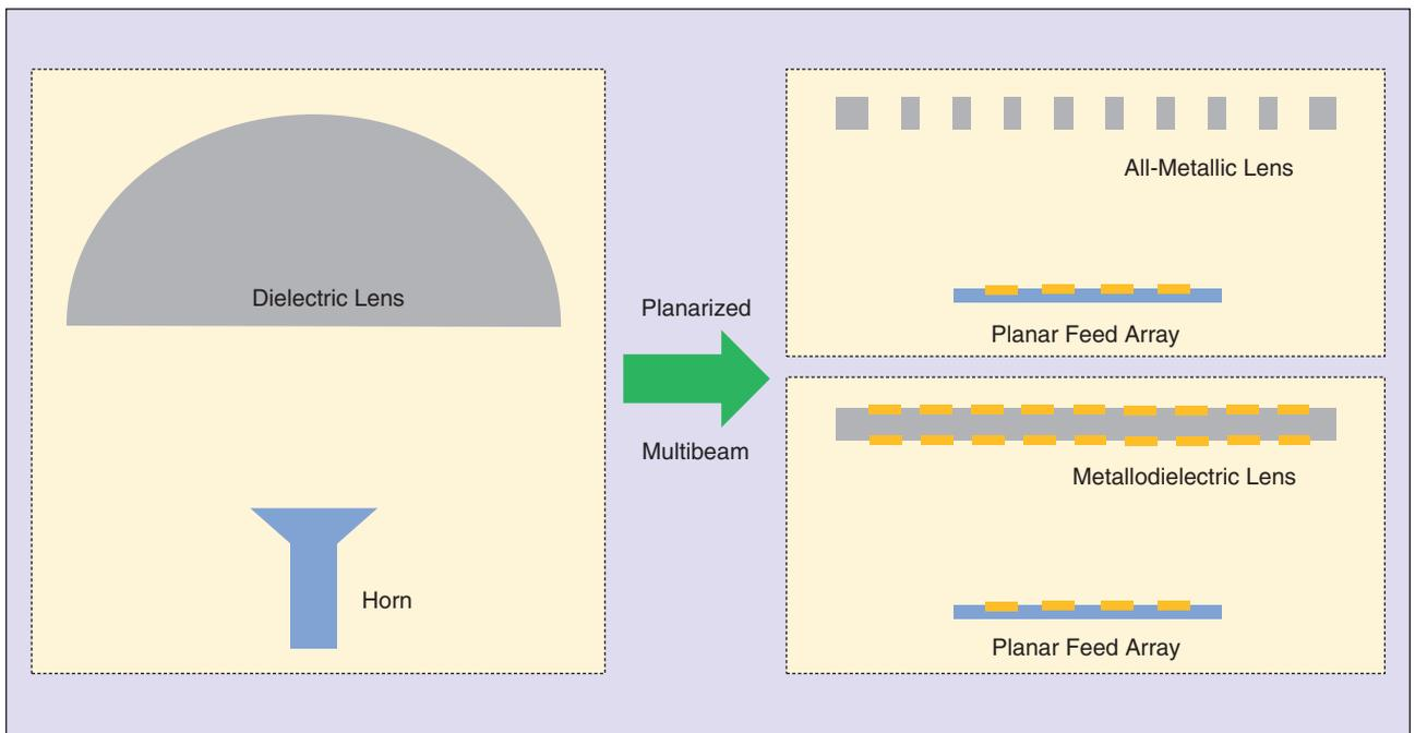
**FIGURE 3** The configuration of THz multibeam antennas using planarized lenses and feed arrays.
