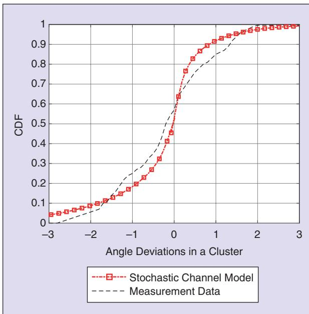
**FIGURE 2** A comparison of the CDFs of angle deviations in a cluster between a stochastic channel model and measurement data. (Source: [4].)
