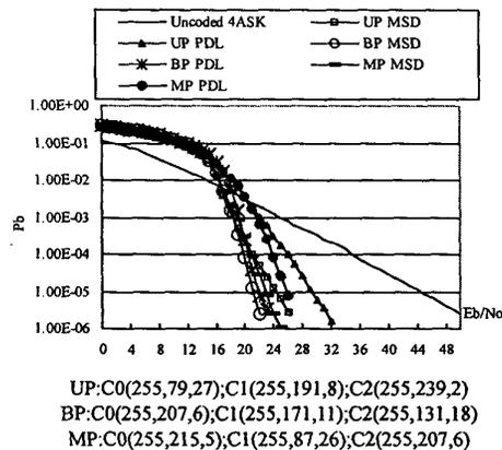
Fig.7 Comparison of MLC/MSD and MLC/PDL with 8ASK, over Rayleigh channel
