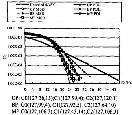
Fig.6 Comparison of MSD and PDL with 8ASK over Rayleigh channel
