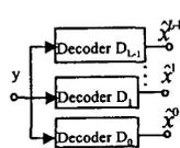
Fig.4 Parallel decoding of levels
