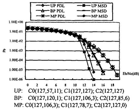
Fig.5 Comparison of MSD and PDL with 8ASK over AWGN channel
