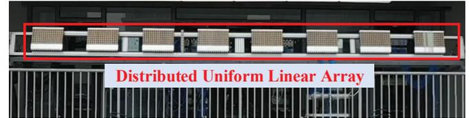
(c) The ultra-massive MIMO antenna configuration with the DULA.
