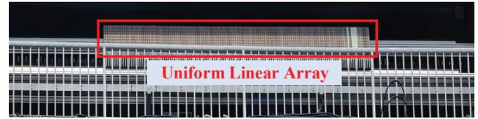
(b) The ultra-massive MIMO antenna configuration with the ULA.
