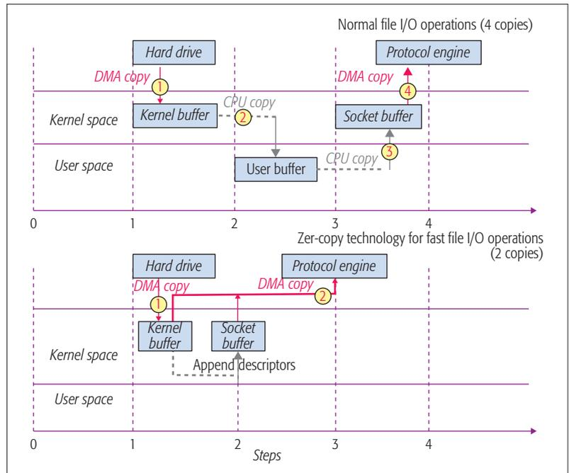
FIGURE 3. Zero-copy technology for high-speed data storage
