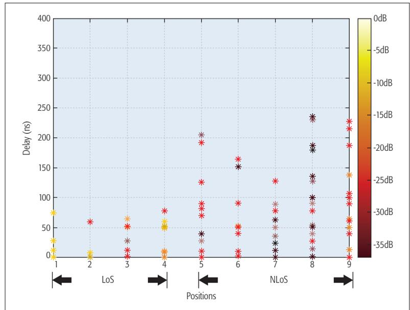
FIGURE 6. Normalized power delay profiles at LoS and NLoS positions.
