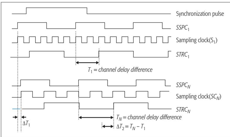
FIGURE 2. Clock phase alignment and synchronization mechanism.
