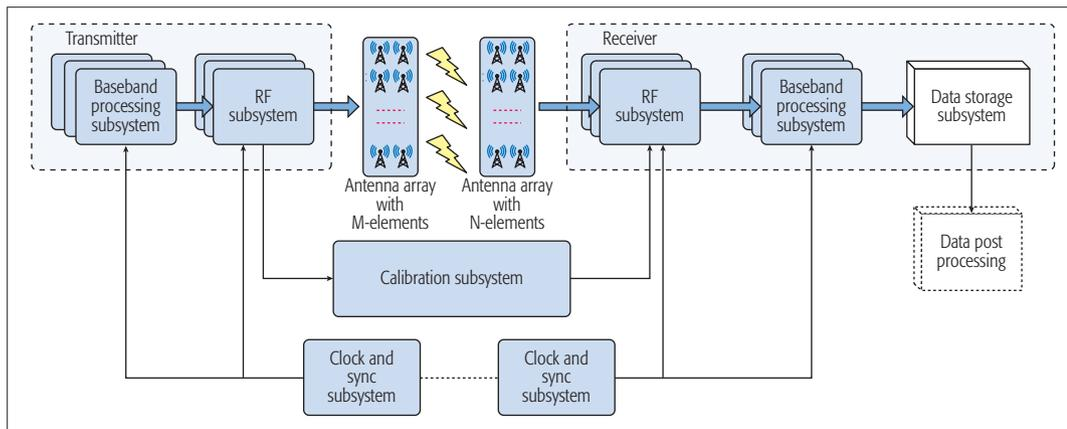
FIGURE 1. System architecture of the MIMO parallel channel sounder.
