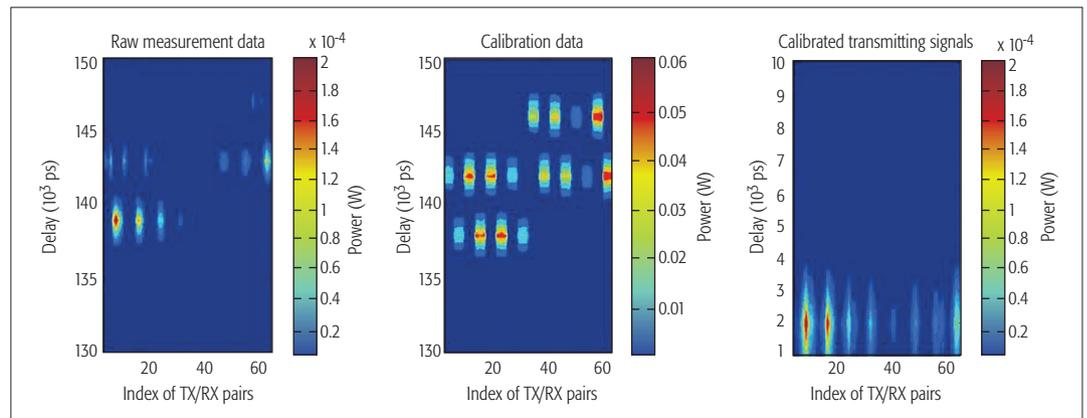
FIGURE 5. Power delay profiles at 64 TX/RX pairs before and after calibration.
