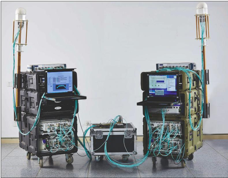
FIGURE 4. Implementation of the MIMO parallel channel sounder.
