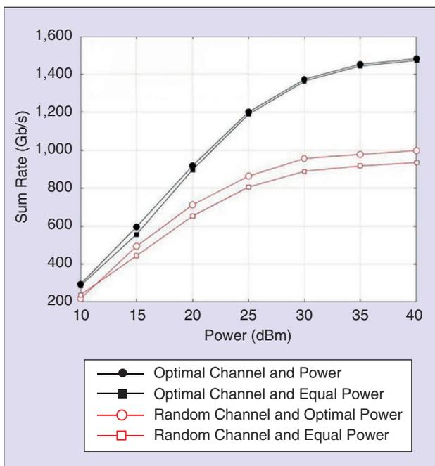
**FIGURE 6** The sum rate versus the transmit power of the access point in a typical WLAN scenario.
