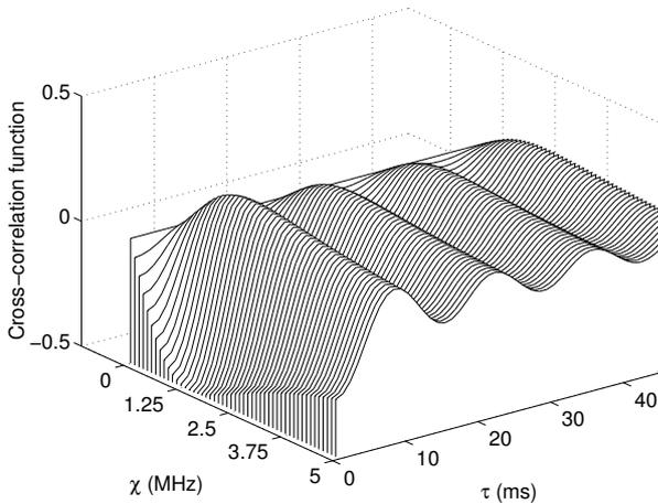
Fig. 4: Cross-correlation function  $r_{\mu_1\mu'_2}(\tau, \chi)$  (ref. model) for the COST 207 RA profile ( $\alpha = 0.1086 \mu\text{s}$ ,  $f_{max} = 91$  Hz,  $\sigma_0^2 = 1$ ).
