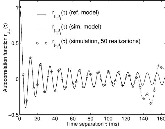
Fig. 1: Autocorrelation function  $r_{\mu_i\mu_i}(\tau)$  (ref. model) in comparison with  $\hat{r}_{\mu_i\mu_i}(\tau)$  (sim. model,  $N = 20$ ,  $M = 20$ ) for  $f_{max} = 91$  Hz and  $\sigma_0^2 = 1$ .
