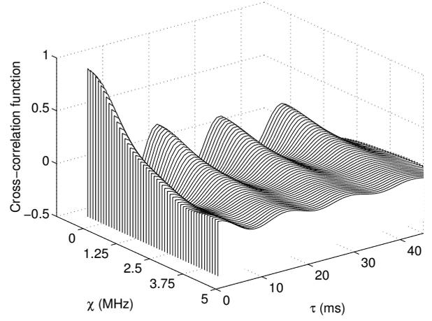
Fig. 3: Cross-correlation function  $\hat{r}_{\mu_i\mu'_i}(\tau, \chi)$  (sim. model,  $N = 20$ ,  $M = 20$ ) for the COST 207 RA profile ( $\alpha = 0.1086 \mu\text{s}$ ,  $f_{max} = 91$  Hz,  $\sigma_0^2 = 1$ ).
