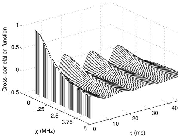
Fig. 2: Cross-correlation function  $r_{\mu_i\mu'_i}(\tau, \chi)$  (ref. model) for the COST 207 RA profile ( $\alpha = 0.1086 \mu\text{s}$ ,  $f_{max} = 91$  Hz,  $\sigma_0^2 = 1$ ).
