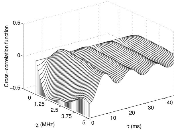
Fig. 5: Cross-correlation function  $\hat{r}_{\mu_1\mu'_2}(\tau, \chi)$  (sim. model,  $N = 20$ ,  $M = 20$ ) for the COST 207 RA profile ( $\alpha = 0.1086 \mu\text{s}$ ,  $f_{max} = 91$  Hz,  $\sigma_0^2 = 1$ ).
