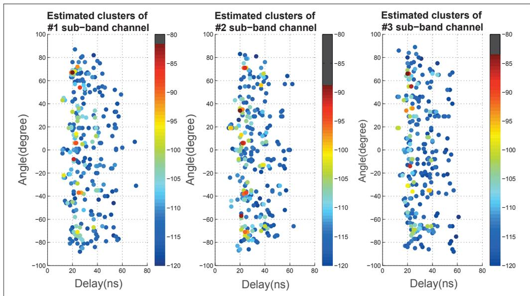
Figure 2. The measured power angular spectrum at different sub-bands.
