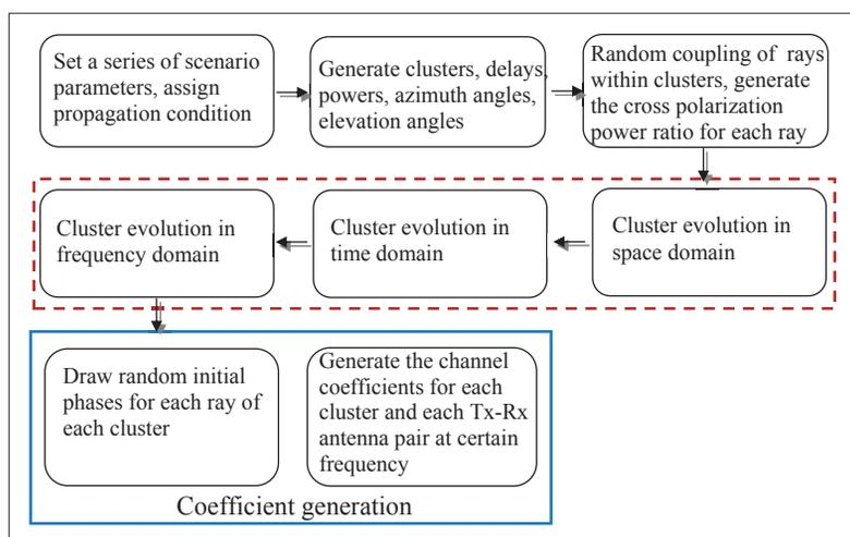
Figure 3. The modeling process of the novel HST channel model.
