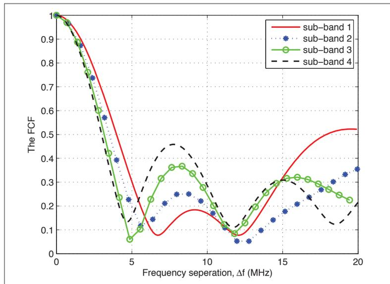
Figure 4. The frequency correlation functions of the mmWave HST channel model at different sub-bands.
