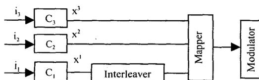
Fig. 1. Improved multilevel coder with intralevel bit interleaver
