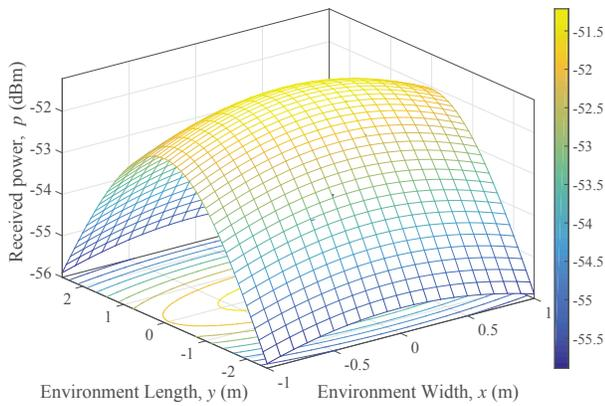
Fig. 6. Power distribution at the miner plane.
