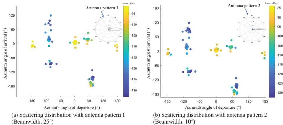
Fig. 3. Scattering distributions with different antenna configurations.
