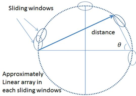
Fig. 4. Approximation of linear antenna subarrays [7].
