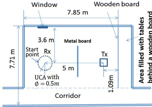
Fig. 3. Floorplan of channel measurements in the basement [7].
