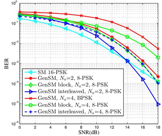
Fig. 6. BER versus the SNR for SM, conventional GenSM, GenSM with block grouping and interleaved grouping with different  $N_a$  for  $N_t = 8$ ,  $N_r = 8$ ,  $\rho = 0.7$ ,  $\eta = 7$ .
