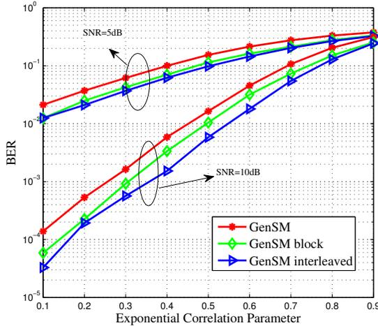
Fig. 5. BER versus the exponential correlation parameter  $\rho$  for conventional GenSM, GenSM with block grouping and interleaved grouping for  $N_t = 16$ ,  $N_r = 8$ ,  $N_a = 2$ ,  $\eta = 7$ , SNR = 5 or 10dB.
