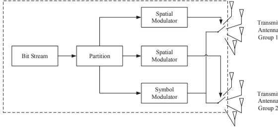
Fig. 1. Block diagram of the transmitter of GenSM with transmit antenna grouping ( $N_t = 8, N_a = 2$ ).
