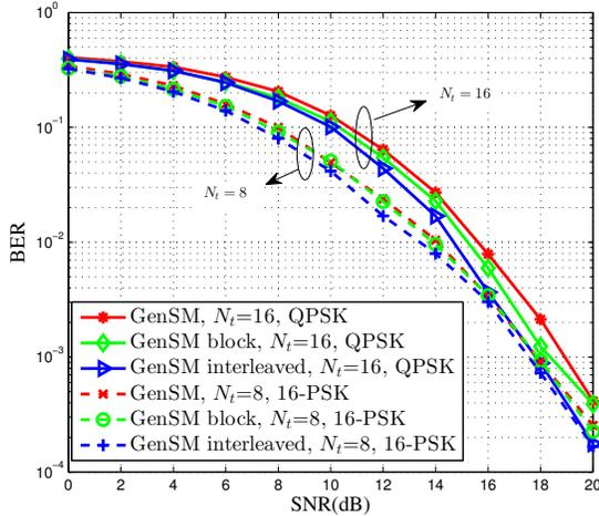
Fig. 7. BER versus the SNR for conventional GenSM, GenSM with block grouping and interleaved grouping with different  $N_t$  in equal size for  $N_r = 4$ ,  $N_a = 2$ ,  $\rho_{16} = 0.5$ ,  $\rho_8 = 0.25$ ,  $\eta = 8$ .
