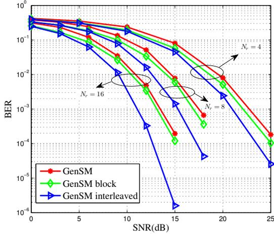
Fig. 4. BER versus the SNR for conventional GenSM, GenSM with block grouping and interleaved grouping with different  $N_r$  for  $N_t = 16$ ,  $N_a = 2$ ,  $\rho = 0.7$ ,  $\eta = 7$ .
