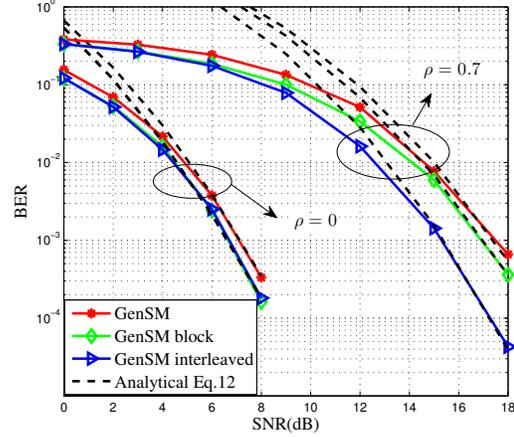
Fig. 3. BER versus the SNR for conventional GenSM, GenSM with block grouping and interleaved grouping for  $N_t = 16, N_r = 8, N_a = 2, \rho = 0$  or  $0.7, \eta = 7$ .
