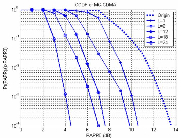
Fig.4. CCDF of PAPR with N=64 and different value of L .
