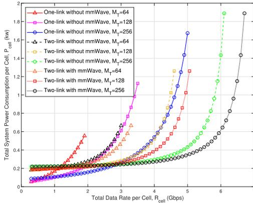
Fig. 6. Comparison of system power consumption at different data rates for one-link and two-link network architectures with and without mmWave technology.
