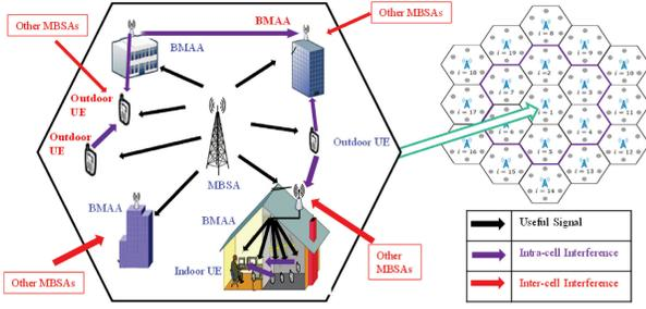
Fig. 1. The system model of a potential B5G wireless network.
