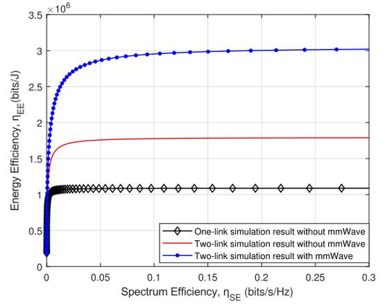
Fig. 7. EE and SE trade-off for one-link and two-link network architectures with and without mmWave technology.
