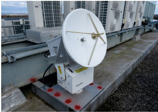
(a) The Alphasat beacon Rx on the top of a building at HWU.
