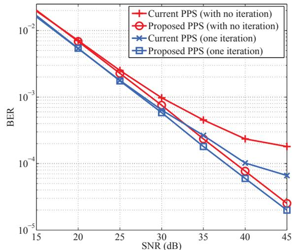
Fig. 4. BER performance comparison between the current PPS and proposed PPS techniques in a Rayleigh flat-fading channel.
