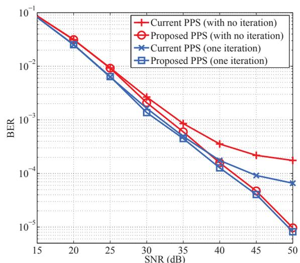
Fig. 5. BER performance comparison between the current PPS and proposed PPS techniques in a frequency-selective Rayleigh fading channel.
