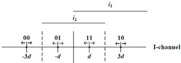
Fig. 2. Signal space diagram for 4-PAM.
