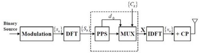
Fig. 1. The block diagram of the transmitter with the FDPMT.
