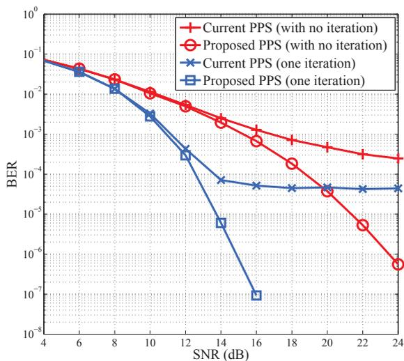
Fig. 3. BER performance comparison between the current PPS and proposed PPS techniques in an AWGN channel.
