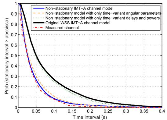
**FIGURE 4. The empirical CCDFs of stationary intervals for the original WSS IMT-A MIMO channel model and the proposed non-stationary IMT-A MIMO channel model with all time-variant parameters, only time-variant delays and powers, and only time-variant angular parameters.**
