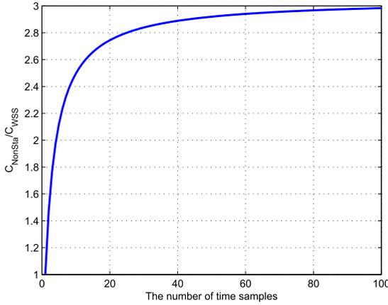
**FIGURE 3. Complexity comparison between the original WSS and non-stationary IMT-A MIMO channel models with different time samples in the considered HST scenario.**
