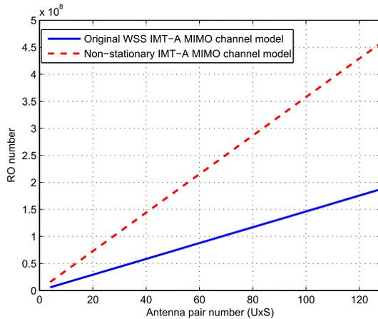
**FIGURE 1.** Complexity comparison of the original WSS and non-stationary IMT-A MIMO channel models with different antenna pair numbers in the considered HST scenario.
