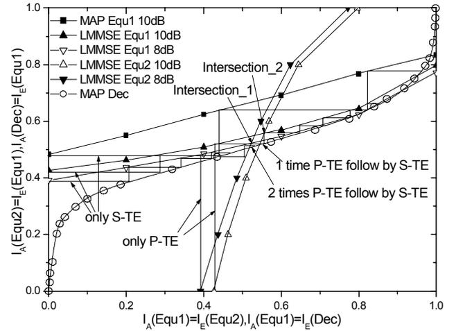
Fig. 5. The EXIT chart of the novel iterative method for the 8PSK modulation ( $M=5$ ).
