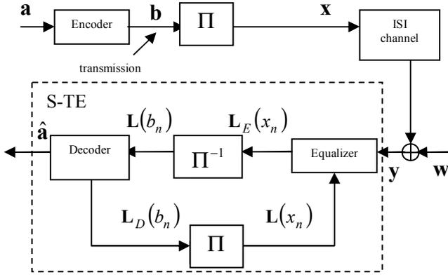
Fig. 1. A coded data transmission system with a S-TE.
