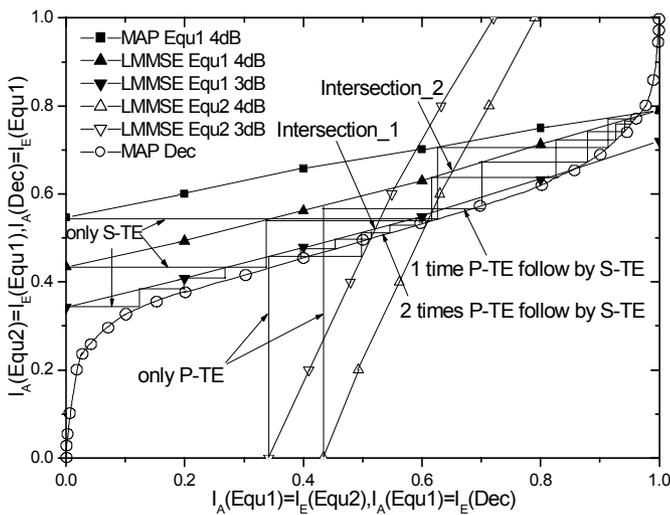
Fig. 4. The EXIT chart of the novel iterative method for the BPSK modulation  $M=3$ .
