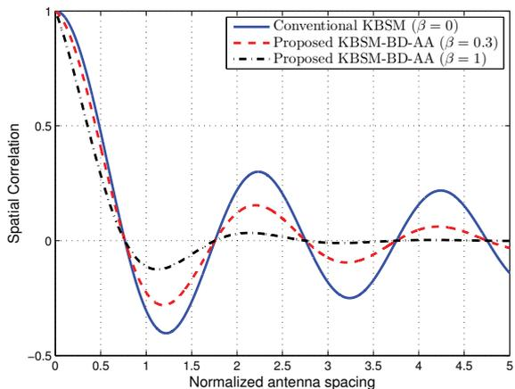
Fig. 3: Antenna spatial correlation for the KBSM-BD-AA (isotropic scattering environment).
