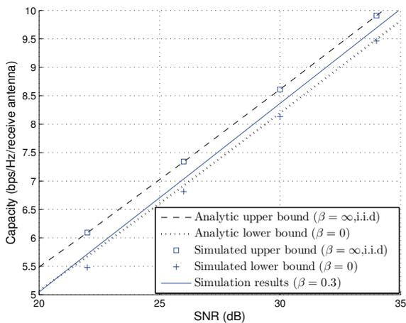
Fig. 5: Capacity analysis in the high SNR regime for the KBSM-BD-AA ( $M_R = M_T = 64$ , half-wavelength ULAs, isotropic scattering environment).
