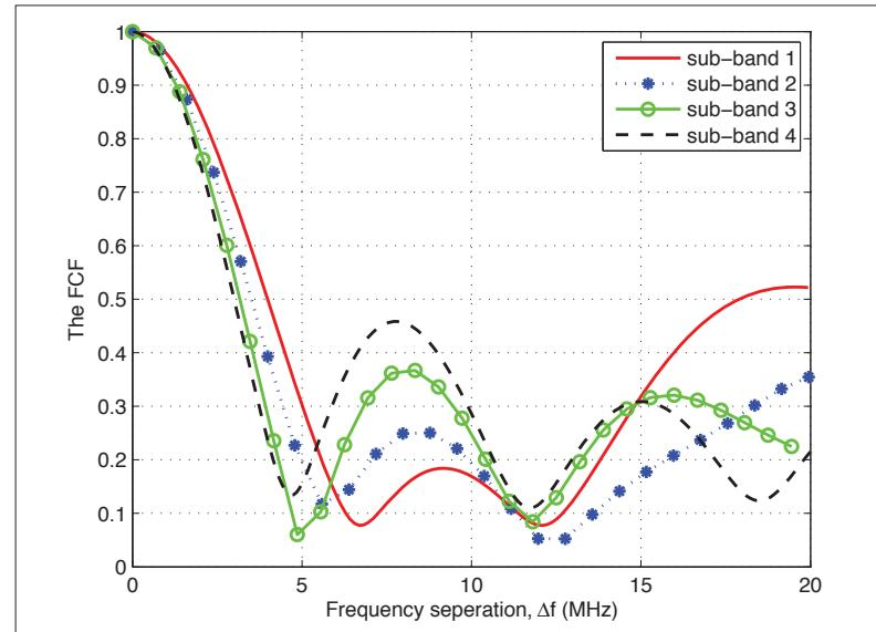
**Figure 4.** The frequency correlation functions of the mmWave HST channel model at different sub-bands.
