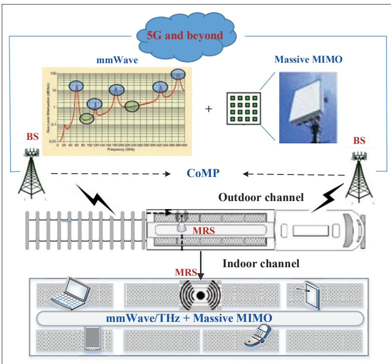
Figure 1. Network architecture for future railway communications.
